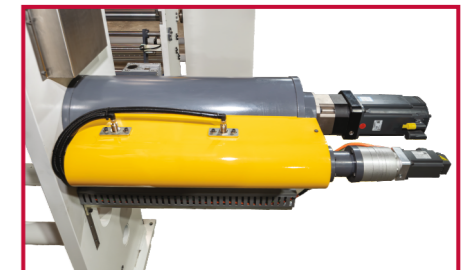
Zero-backlash gear ratio for better print registration
